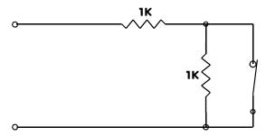
This circuit provides a high degree of supervision and detects both short and open circuit fault conditions. Use this circuit in high security applications.
