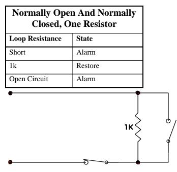
This circuit type is used where normally open and normally closed contacts are used in the same loop.
