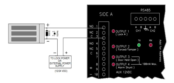
For magnetic locks, the relay should be configured from the PC as normally energized for fail-safe operation. If power fails (*AC and battery*) or the fire input is released, the power to the magnetic lock is removed and the door is opened.
