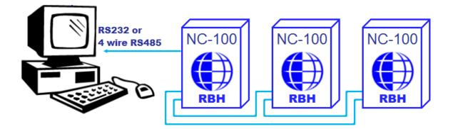
The controllers are wired together in a high-speed fault tolerant ring network. Fault tolerance means the system is immune to a single point of failure and will continue to operate with a short or cut on any single cable section. The fault condition is reported to the PC.
