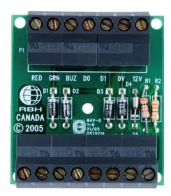
Our EXITRDR Exit reader module is a flexible, convenient and inexpensive way to control and track cardholder access in both directions through the same door.
